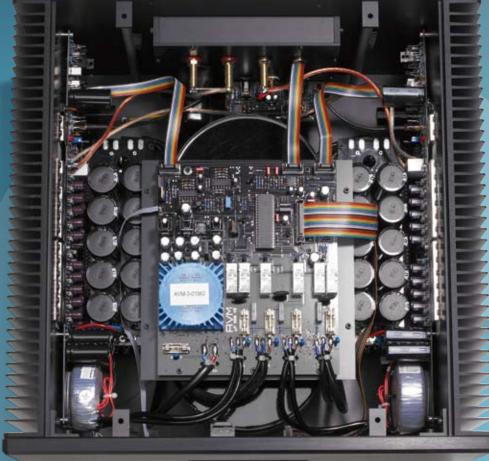
So much beauty for just one channel: The MA8.2 is a bridge amplifier with individual supplies for each signal half. Thus, we find two 1000 VA toroids and electrolytics with a total capacity of 400,000 pF in each monobloc. The input stages have their own small toroids at the front left and right corners. The blue transformer on the top board powers the standby and control circuitry.
