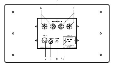
5, 6: **Speaker connectors** 8: **RCA-Cinch input** 10: Power supply socket 7: **Balanced input**
