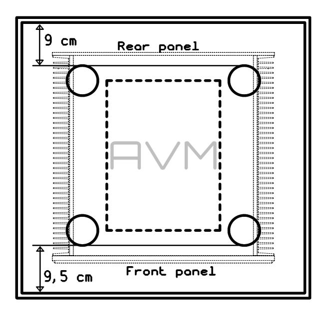
NOTE: if the unit is not positioned in the correct direction the cover will not fit exactly. In this case turn the unit by 180 degrees.
